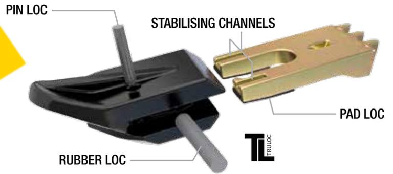
Digga's new TRULOC tooth range allows the tooth to be secured in 3 different ways; Use 1, use 2, or use them all. The range also features an easy-to-remove pin, stabilising channels and the Digga quality that you've come to expect. The TRULOC tooth comes in three models for various ground conditions; earth (E) - for soft ground, flat tungsten (TC) - for medium to hard ground, and multi-facet tungsten (MFT) for tougher ground conditions.
